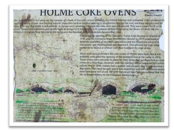
Relatively little is known about the coke ovens, but the most likely reason for their existence here is to provide coke to iron works in the area. Coke is derived from coal and is preferred in iron and steel manufacture because the impurities such as sulphur which are present in coal have been removed by heating in the absence of air – this makes the resulting iron purer and therefore stronger.
